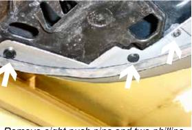
2. Remove eight push pins and two phillips screws from the lower back edge of fascia.
