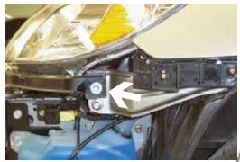
Remove the metric bolt from headlight assembly with the 10MM socket, pull forward, unplug electrical and set aside, both sides.
