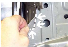
**12.** Cut and remove forward webbing on lower frame with the hack saw or reciprocating saw, both sides.
