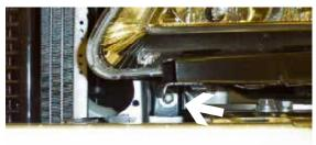
**5.** Remove one metric bolt from below headlight assembly with the 10MM socket, both sides.
