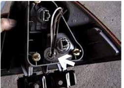
Location for the BX8869, bulb and socket on the driver's side of the 2004 model.
