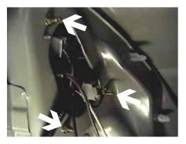
Remove two push pins from trunk liner. Pull liner back and remove three metric nuts from taillight assembly with the 8MM socket (left photo). Remove one phillips screw on the bottom of taillight assembly bracket from under the rear fascia (right photo).
